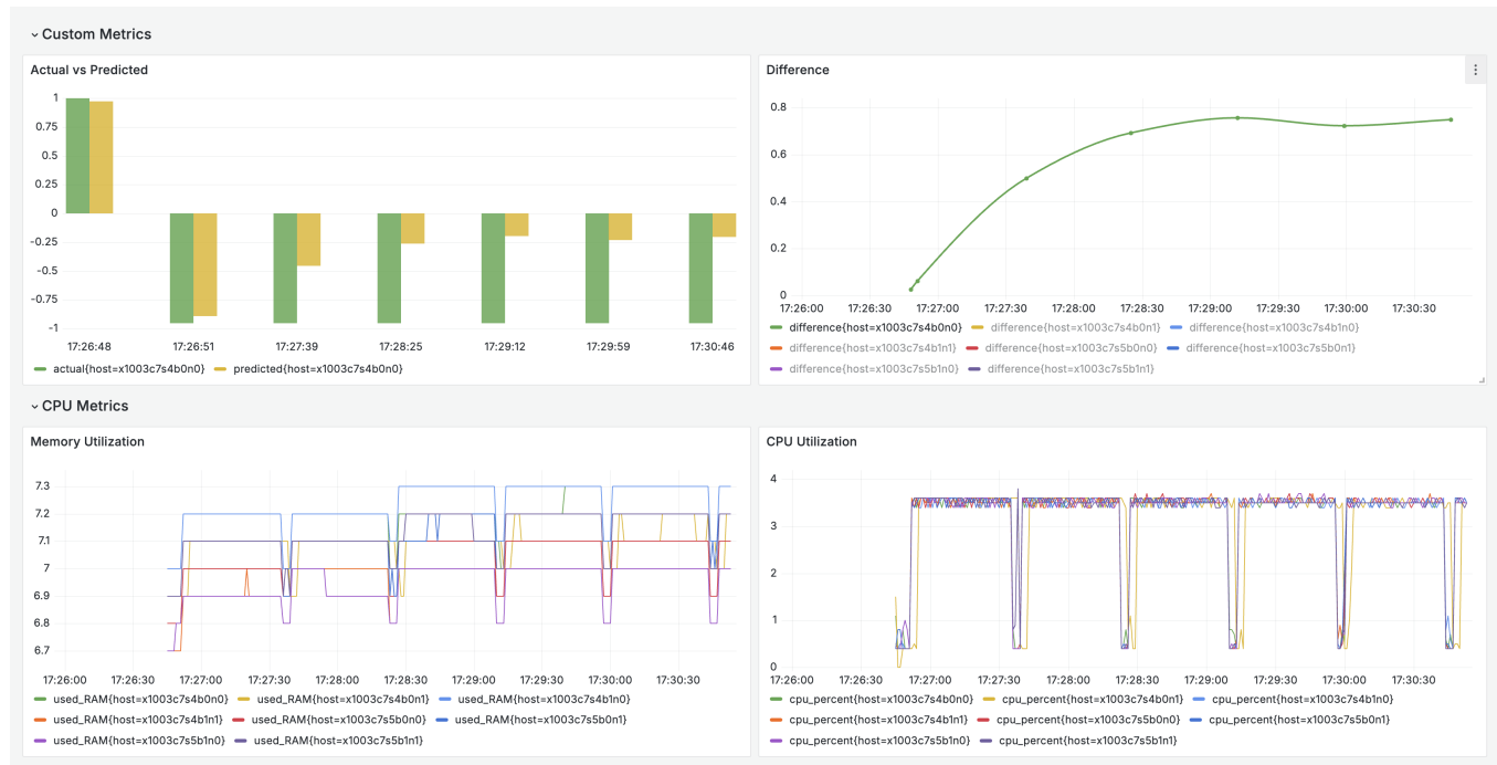
Figure 3: Grafana dashboard with Dragon Telemetry Service metrics
